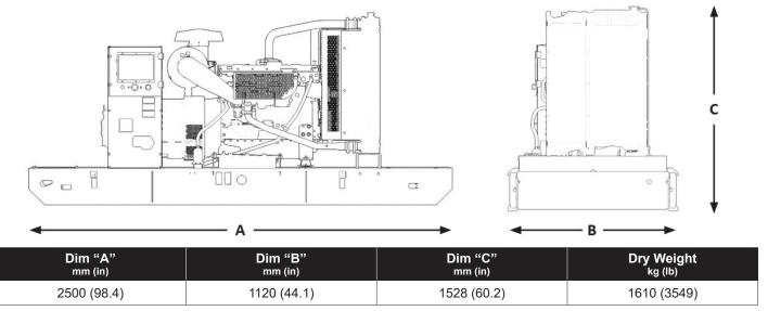
Note: General configuration not to be used for installation. See general dimension drawings for detail.
