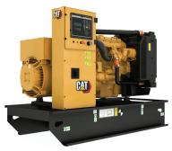
Engine ModelCat® C4.4 Inline 4-stroke DieselBore x Stroke105.0mm x 127.0mm (4.1in x 5.0 in)Displacement4.4 L (268.4 in³)Compression Ratio16.7:1AspirationTurbocharged Air To Air Charge CooledFuel Injection SystemInlineGovernorElectronic
