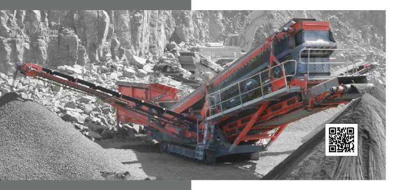
The Finlay<sup>®</sup> 693+ Spaleck is the ultimate in mobile fine screening and separation technology. At the heart of the plant is an innovative 2-deck German designed and constructed high performance aggressive screenbox with state of the art flip flow technology on both the top and bottom decks.
