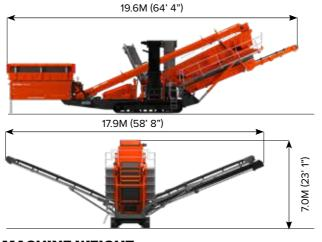
MACHINE WEIGHT: 40,000KG (88,184LBS) (WITH TIPPING GRID)
