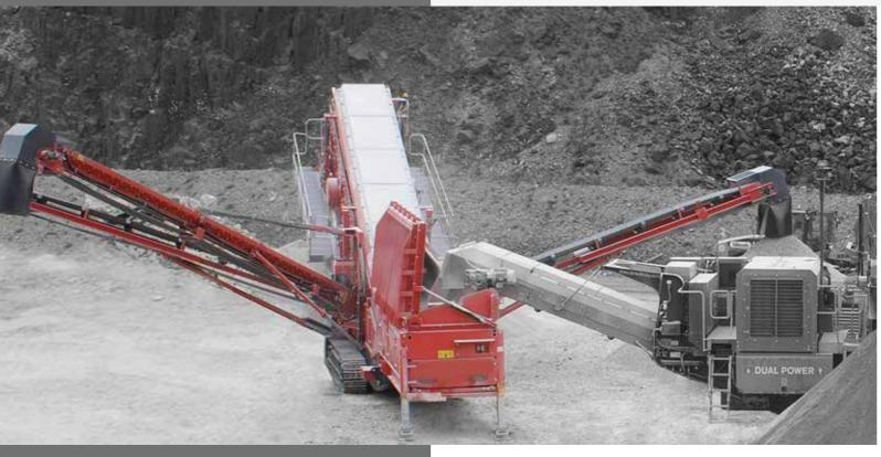
The Finlay<sup>®</sup> 694+ Hybrid Inclined Screen offers operators the flexibility to power the plant either by an electrical connection or diesel/hydraulic configuration. The plant features a triple deck screen configuration providing three full sized 6.1m x 1.53m (20' x 5') screens.
