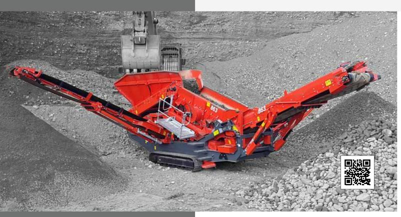
The Finlay® 863+ mobile scalper is a compact and aggressive forward facing screen. This flexible and mobile plant can work in aggregates, sand and gravel, top soil, construction demolition and recycling applications where site space is at a premium.
