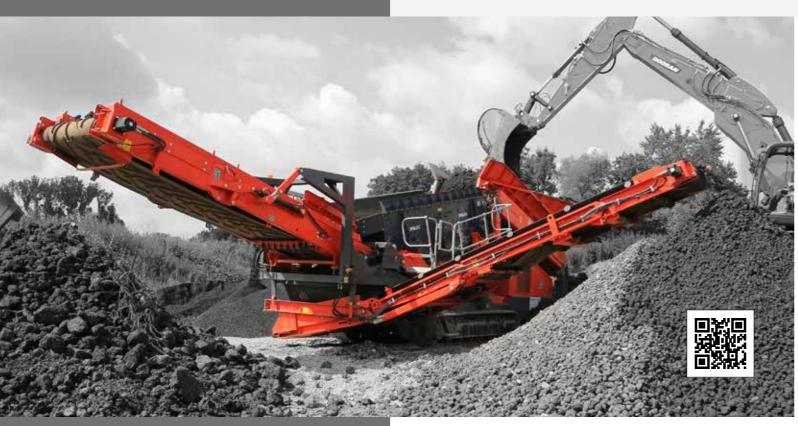
The Finlay® 873+ Spaleck is a mobile scalper ideally suited to working in aggregates, sand and gravel, top soil, construction demolition and recycling applications. This highly versatile machine can be fed either by a tracked mobile crusher, shovel or an excavator.
