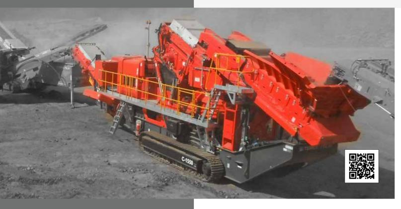
The Finlay® C-1550P incorporates the proven Terex® 1300 cone crusher driven through direct drive.
