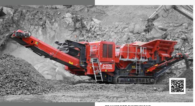
The Finlay® J-1175 hybrid mobile jaw crusher offers operators the flexibility to power the plant either by mains electric connection or the onboard genset powerpack configuration.
