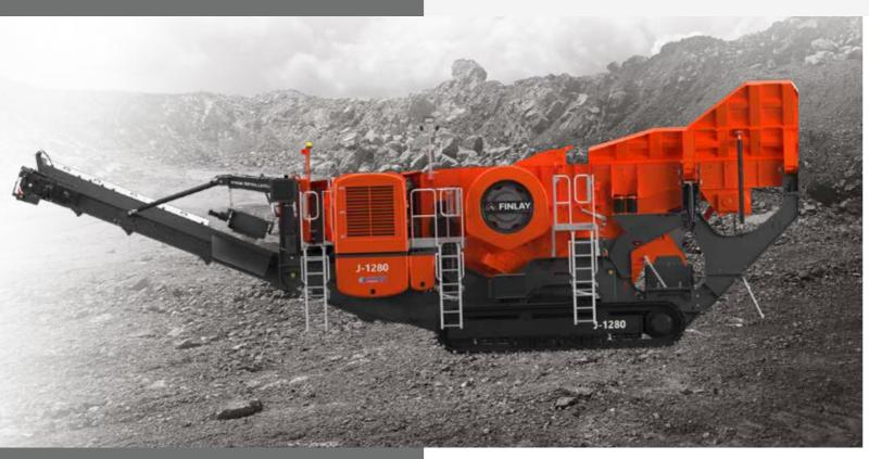
The Finlay® J-1280 hybrid mobile jaw crusher offers operators the flexibility to power the plant either by an onboard genset powerpack configuration or connected to an external power source. Both power options provide operators with significant power, servicing and maintenance cost savings in direct comparison to a diesel/hydraulic powered plant.
